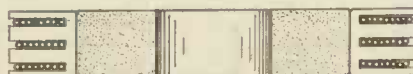
Fig. 2—Iron core loop antenna of this design may have Q of 500 to 600
