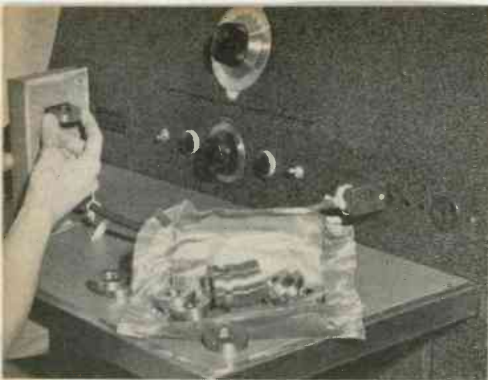
Using the Cyclograph to check the case-hardening depth of roller bearings
