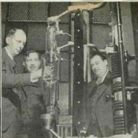
Millionth-second Westinghouse tube can X-ray in-thick armor plate as projectile tears through
