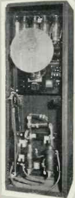
5 SEAM WELD TIMER with roller electrodes uses synchronously driven disc. Provides "On" and "Off" intervals.
