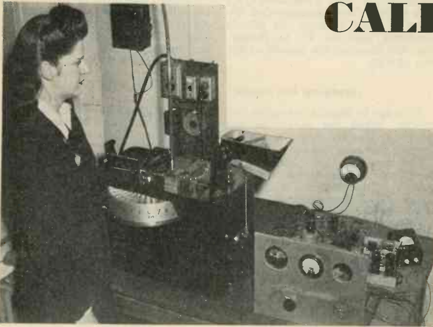
An ingenious electronic control rotates the slotted drum to receive springs automatically measured to close tolerance
