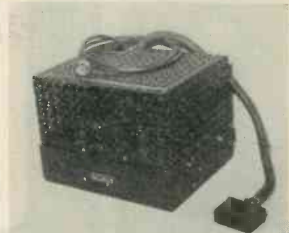
Power supply is arranged for line operation or batteries
