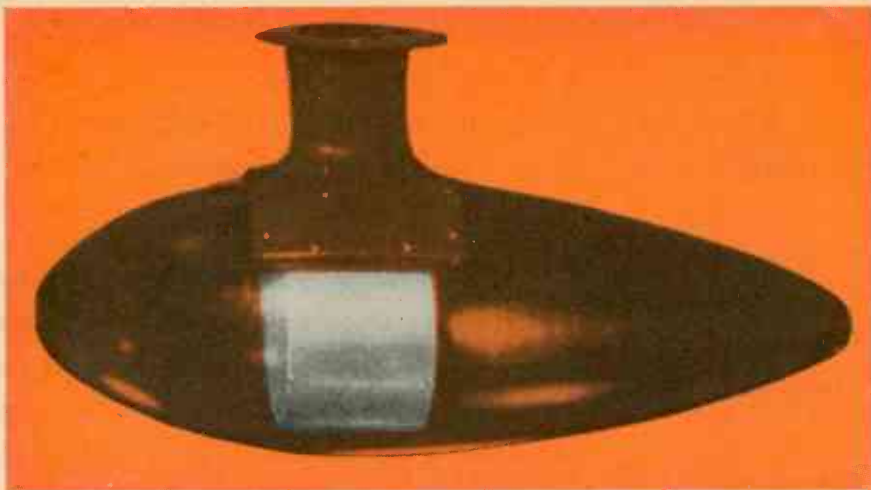
Fig. 1—Relative dimensions of streamlined housing for typical loop antenna as used in modern aircraft design. Housings for iron core loops may be considerably smaller
