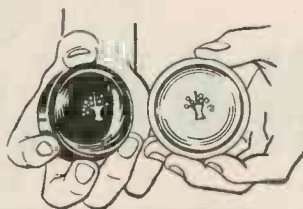
Fine detail easily recorded in the alloy sprayed onto pattern.
