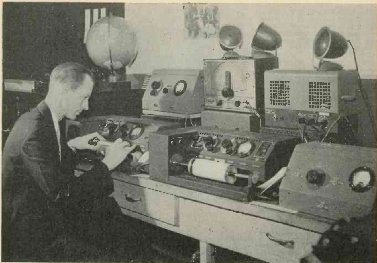
The radio picture equipment used by OWI in various foreign outposts, and here shown in complete form as used at New York headquarters, is compact, easily portable and ready for operation, weighs 45 lbs.
