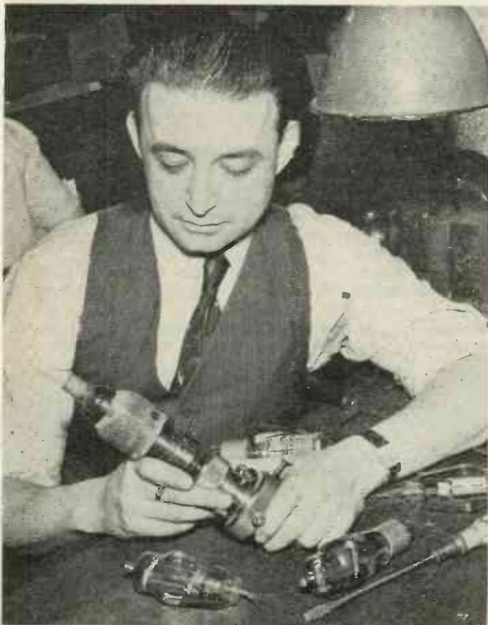
7. TUBE PRODUCTION boosted by collar-like device which holds tube mount while bulb is sealed. Ball bearings and three metal jaws make for easy removal after operation
