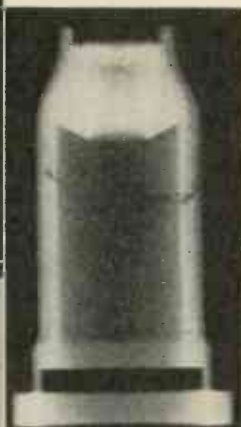
High voltage pressure-molded insulator rejected for defect which might carbonize in service
